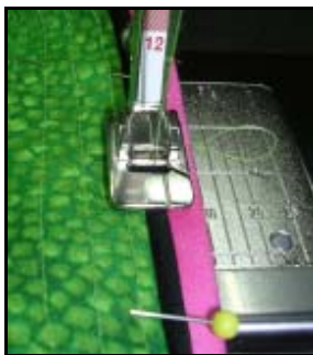
Place the piping in the tunnel under the foot
